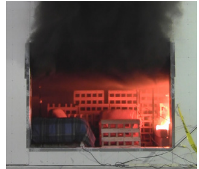
Ignition of the combustible load © Photo: Nordic Structures
