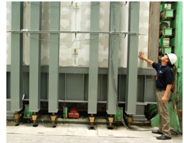
Typical wall after two-hour fire resistance test, temperature over 1,000 °C © Photo: Nordic Structures
