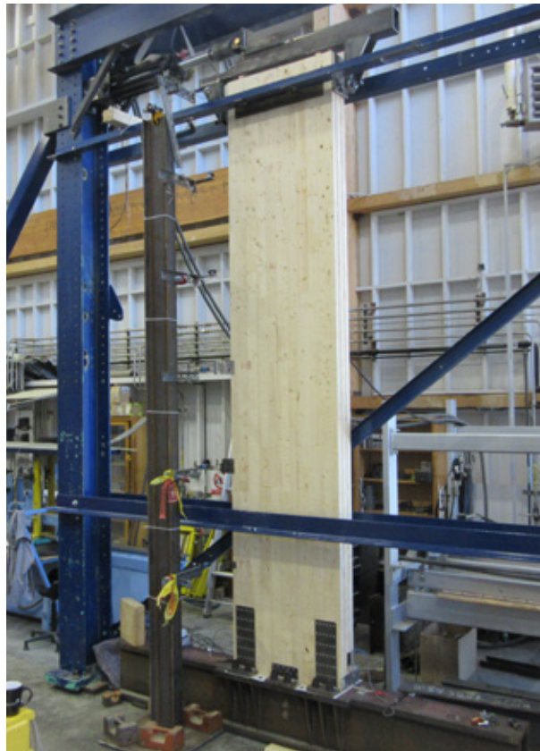
Shear wall testing at FPIinnovations © Photo: FPIinnovations
