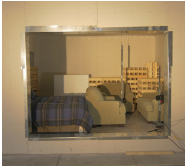
Fire load equivalent to the 95 th percentile of residential fire load density © Photo: Nordic Structures
