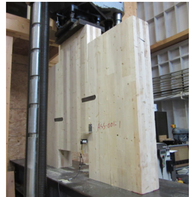
Inserting shear keys in a shear wall and tests at FPIinnovations © Photo: FPIinnovations
