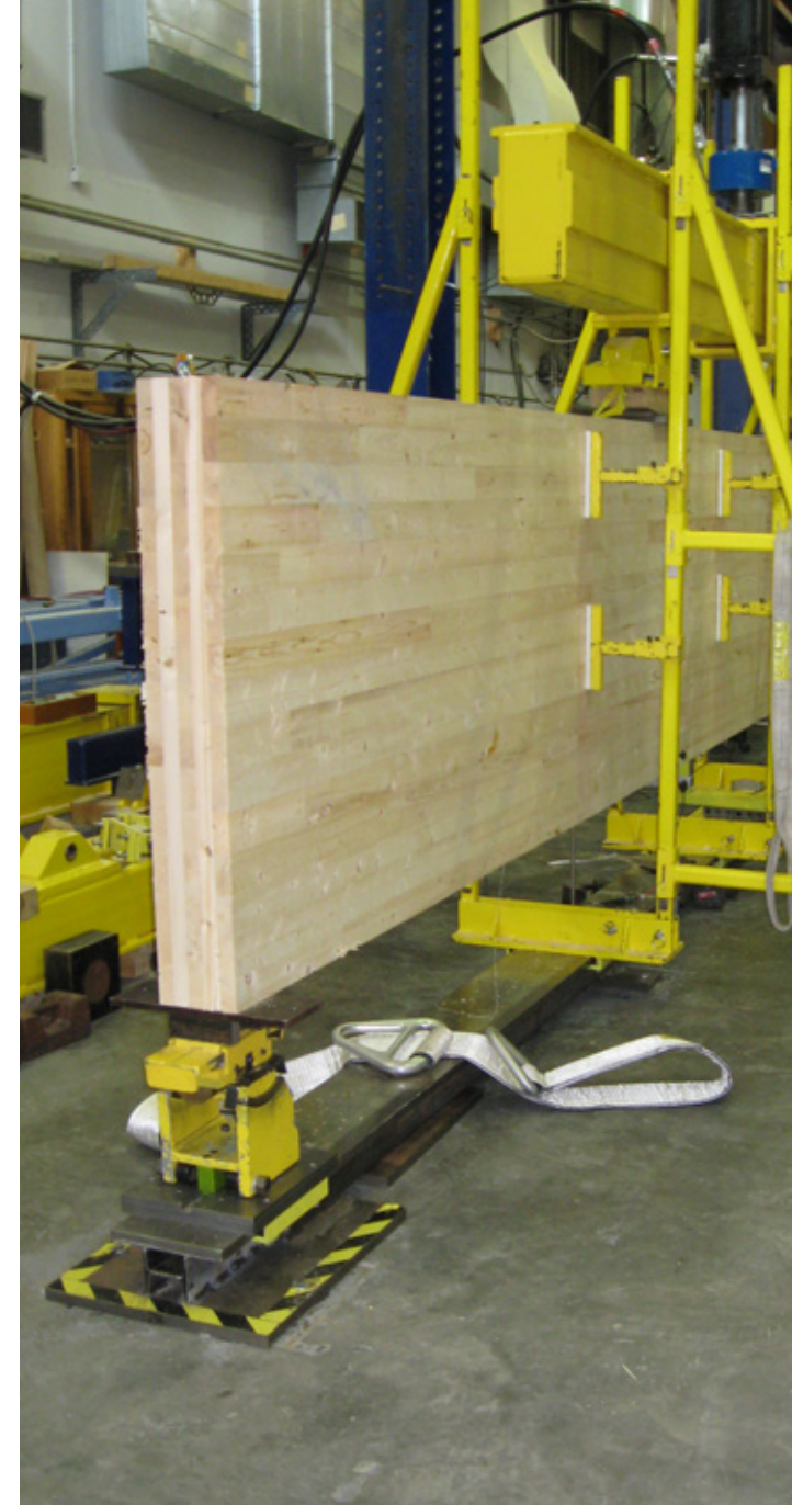
Resistance tests on CLT elements at FPIinnovations © Photo: FPIinnovations
