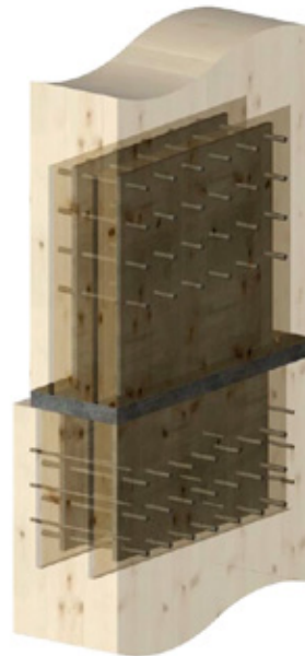
Junction steel plate to vertically connect the shear wall CLT panels © Photo: Stéphane Groleau
