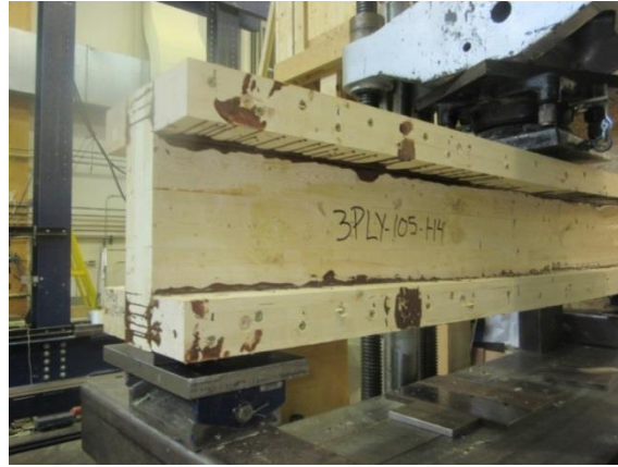
Figure 3 – Reinforced CLT Beam with glulam at FPIinnovations' Lab in Québec
