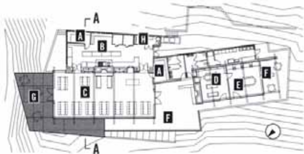
Dining hall plan A Storage D Library G Deck B Kitchen E Conference room H Mechanical C Dining F Terrace
