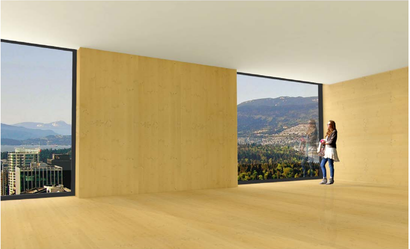
Interior perspective illustrating structure as finishing
