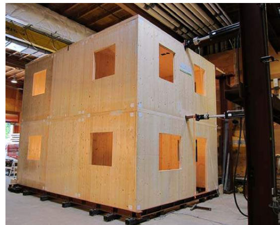
2 Storey CLT Structure Testing FPInnovations
