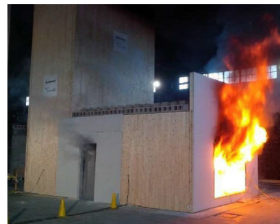
Fire Shaft 2hr Test: No sign of smoke or heat penetration into the shaft.
