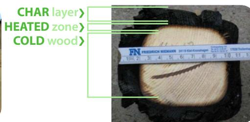
The unburnt wood, protected by the charred wood, retains up to 100 percent of its initial strength.
