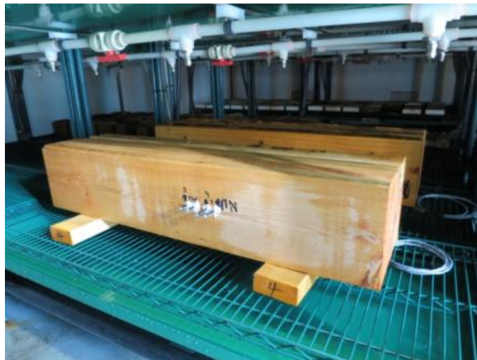
Figure 4 Nail-laminated timber specimens being wetted by controlled spray of water in the laboratory
