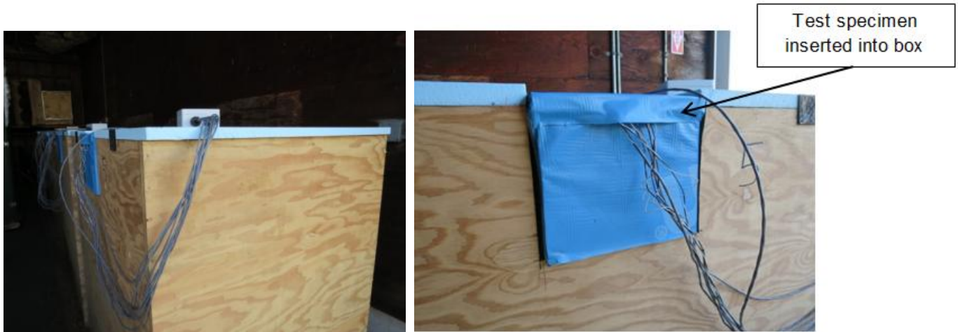
Figure 6 Nail-laminated timber assemblies undergoing drying above plywood boxes in the shed
