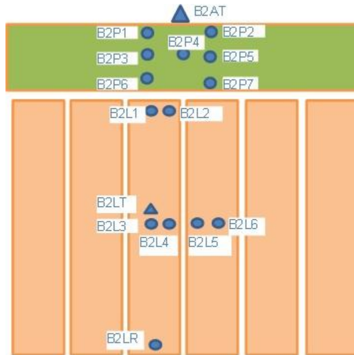
Figure 2 Sensors in central cross section of nail-laminated timber and plywood sheathing as installed in test assembly B2 of Group 3
