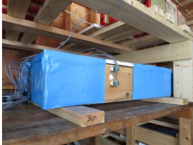
Figure 5 Nailed-laminated timber assemblies undergoing drying in the shed after laboratory wetting
