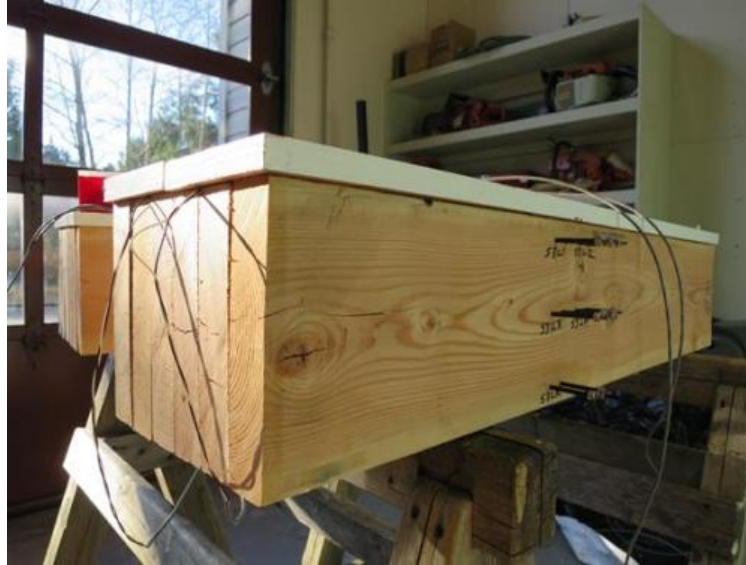
Figure 1 A nail-laminated timber assembly being instrumented in the laboratory
