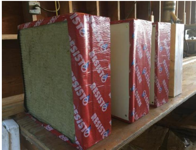
Figure 15. CLT specimens with gypsum board or mineral wool drying in shed [70]
