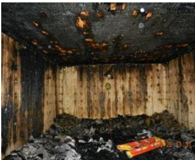
e) Test 1-4 charring of compartment
