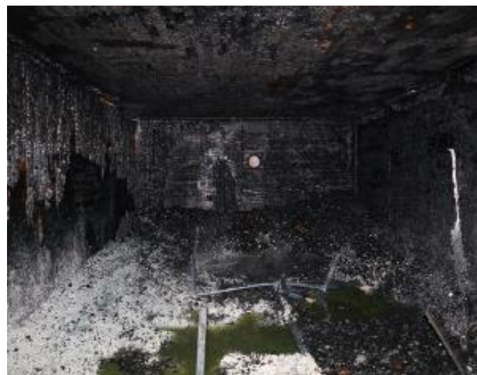
f) Test 1-5 charring of compartment
